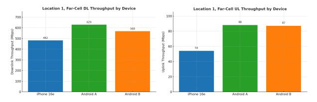
Android A outperformed the iPhone 16e by ~30.5% on DL and 63% on UL in far-cell conditions. Android B exceeded iPhone 16e by ~17.8% on DL and ~61% on UL, performing slightly below Android A but still significantly better than the iPhone 16e.
