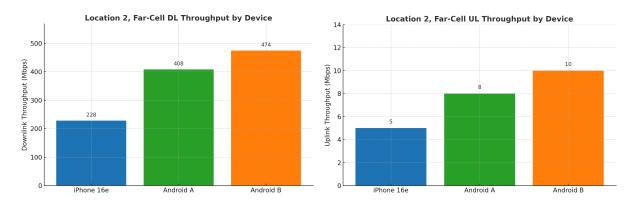
Android A delivers ~79% higher DL and 60% higher UL throughput compared to the iPhone 16e under far-cell conditions. Android B delivers ~108% higher DL and 100% higher UL throughput than the iPhone 16e in the same far-cell scenario. This 1.6X - 2X difference in UL performance has a significant impact on user experience for indoor coverage such as voice and video calls. The last year's
