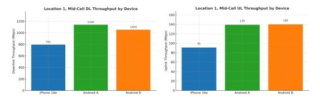
Android A outperformed iPhone 16e by ~43% on DL and ~53% on UL in mid-cell conditions. Android B exceeded iPhone 16e by ~33% on DL and ~54% on UL, again showing strong uplink advantage.
