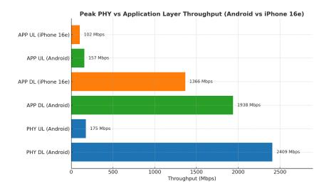
These differences potentially highlight the performance limitations of the Apple C1 modem, particularly in aggregation flexibility and uplink handling, even when network-side constraints are present.
