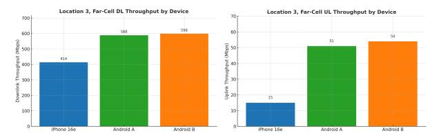
Android A outperformed the iPhone 16e by ~42% on DL and 240% on UL—more than triple the uplink performance. Android B exceeded iPhone 16e by ~44% on DL and a striking 260% on UL, showing nearly quadruple the uplink performance with the DL 4CC CA and ULCA capabilities on full display.
