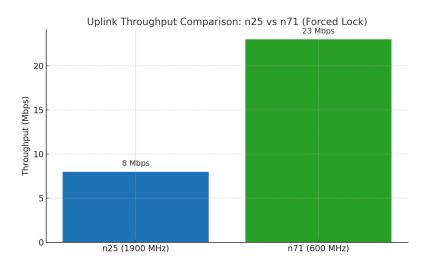
Uplink throughput comparison chart showing the performance difference when locking the device to n25 versus n71. As shown, throughput increased nearly 3x when using n71 under the same far-cell physical conditions.
